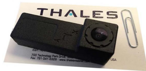
Figure 1: InertiaCam monocular vision-inertial sensor module
